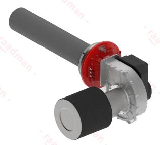
Thanks to standard mixing venturis, gas and combustion air are completely mixed before the fan wheel. Using the PWM pulse and, as a consequence, controlling the rotation of blower, the mixture is transferred to combustion area. Finally, a well spark, leads to a pre-mixed flame with minimum pollution.
