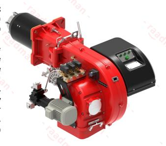
Gas train includes filter, regulator, main and safety valves, pressure gauges, minimum pressure switch, leak test pressure switch, and valve proving system for burners with a capacity of over than 1.2 MW (All according to BS-EN 676).
