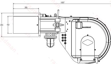
Suggested boiler flange diameter = 205 mm
