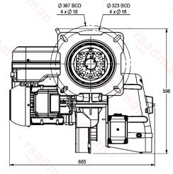
Suggested boiler flange diameter = 235 mm
