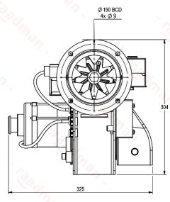
Suggested boiler flange diameter = 133 mm
