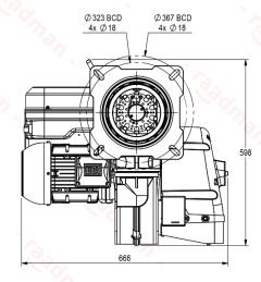
Suggested boiler flange diameter = 235 mm
