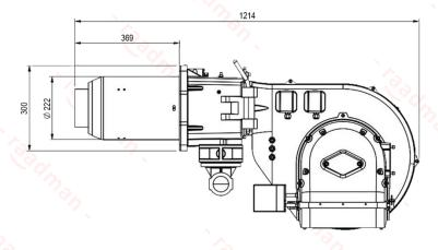
Suggested boiler flange diameter = 336 mm
