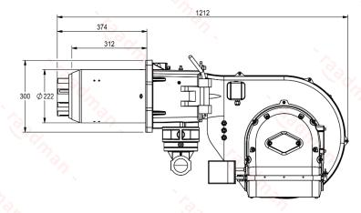
Suggested boiler flange diameter = 336 mm
