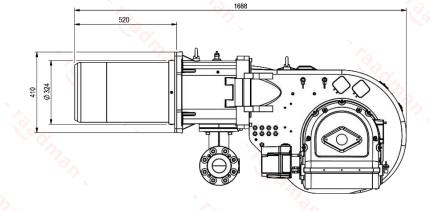
Suggested boiler flange diameter = 335 mm
