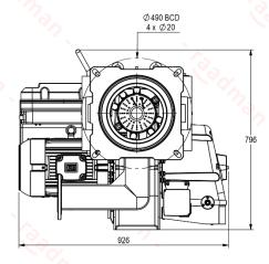
Suggested boiler flange diameter = 335 mm
