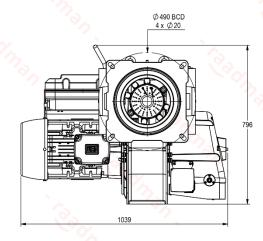
Suggested boiler flange diameter = 335 mm
