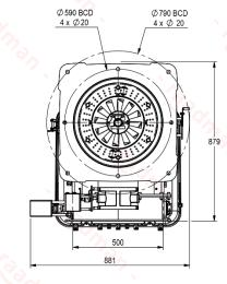
Suggested boiler flange diameter = 495 mm
