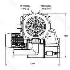
Suggested boiler flange diameter = 495 mm
