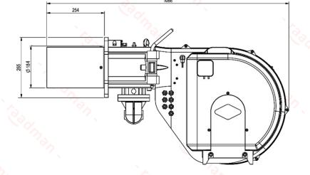
Suggested boiler flange diameter = 192 mm
