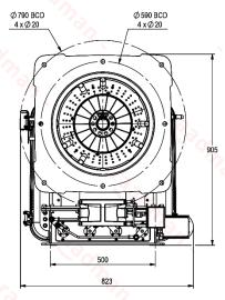
Suggested boiler flange diameter = 605 mm
