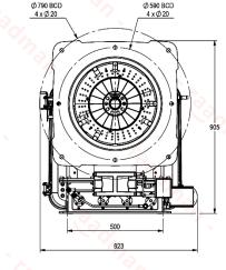
Suggested boiler flange diameter = 492 mm
