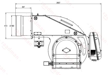
Suggested boiler flange diameter = 492 mm
