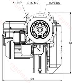
Suggested boiler flange diameter = 201 mm
