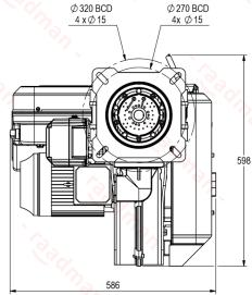
Suggested boiler flange diameter = 201 mm
