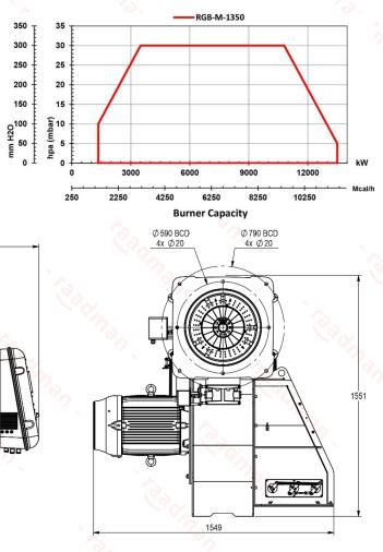
Suggested boiler flange diameter = 492 mm
