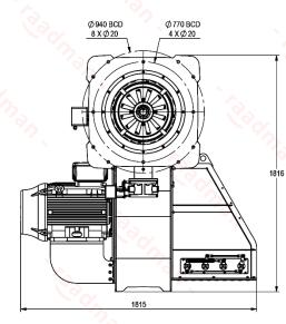
Suggested boiler flange diameter = 602 mm
