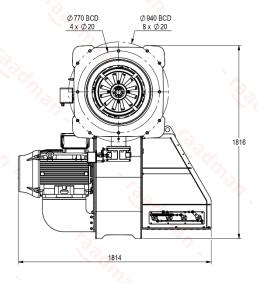
Suggested boiler flange diameter = 620 mm
