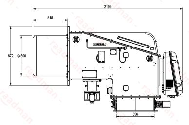
Suggested boiler flange diameter = 605 mm
