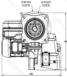
• Suggested boiler flange diameter = 235 mm
