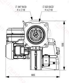
Suggested boiler flange diameter = 235 mm
