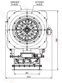
Suggested boiler flange diameter = 605 mm
