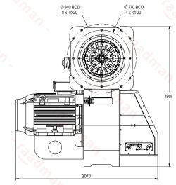
Suggested boiler flange diameter = 620 mm
