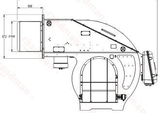
Suggested boiler flange diameter = 620 mm
