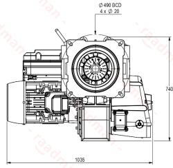
Suggested boiler flange diameter = 335 mm
