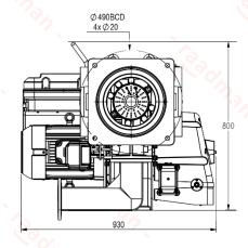
Suggested boiler flange diameter = 336 mm
