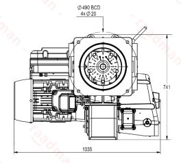
Suggested boiler flange diameter = 343 mm
