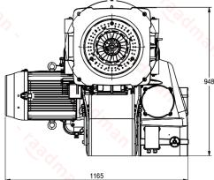
Suggested boiler flange diameter = 415 mm
