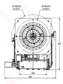
Suggested boiler flange diameter = 415 mm
