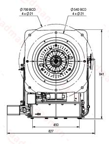
Suggested boiler flange diameter = 426 mm
