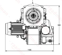
Suggested boiler flange diameter = 415 mm
