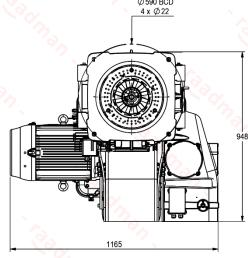
Suggested boiler flange diameter = 415 mm
