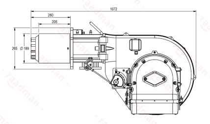
Suggested boiler flange diameter = 201 mm
