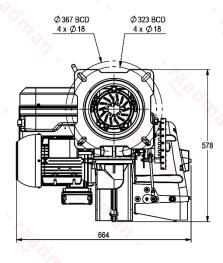
Suggested boiler flange diameter = 234 mm
