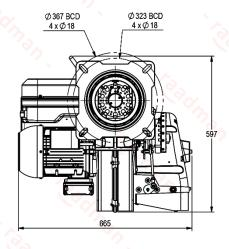
Suggested boiler flange diameter = 235 mm
