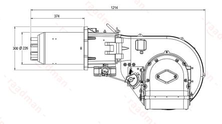
Suggested boiler flange diameter = 235 mm
