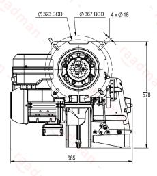
Suggested boiler flange diameter = 235 mm
