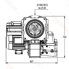
Suggested boiler flange diameter = 335 mm
