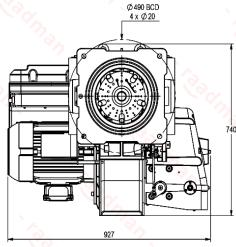
Suggested boiler flange diameter = 336 mm
