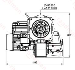
Suggested boiler flange diameter = 337 mm
