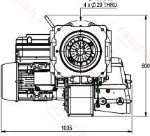
Suggested boiler flange diameter = 337 mm
