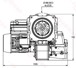
• Suggested boiler flange diameter = 342 mm
