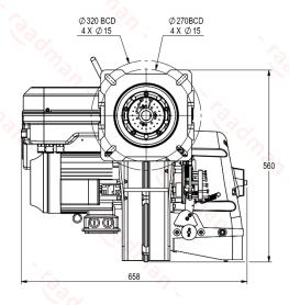
Suggested boiler flange diameter = 201 mm
