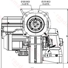
Suggested boiler flange diameter = 201 mm
