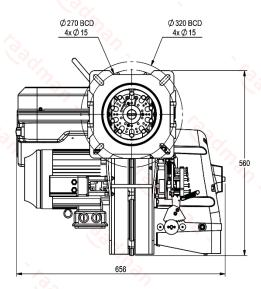
Suggested boiler flange diameter = 202 mm
