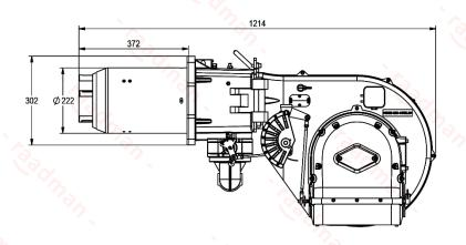
Suggested boiler flange diameter = 234 mm
