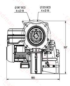
Suggested boiler flange diameter = 235 mm
